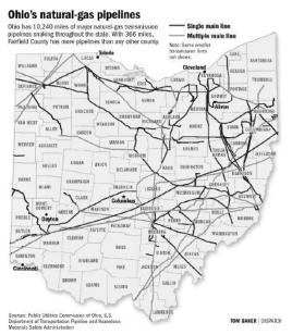
Figure 27: Ohio's Natural-Gas Pipelines Source: Public Utilities Commission of Ohio, US
